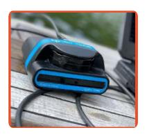
Oculus Multibeam Imaging SONARs are a new generation of compact imaging sonar, designed for use across a wide variety of underwater applications. Their small form factor makes them ideally suited for deployment from micro-sized platforms, while their rugged construction also makes them an excellent choice for work-class vehicles and subsea infrastructure.
